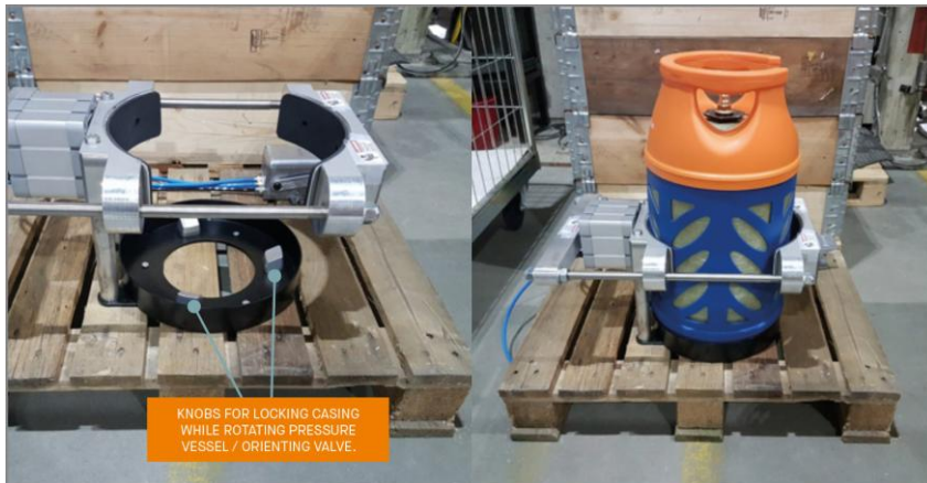
Picture 5-2 Example of casing locking knobs for valve orientation (cylinder clamping not engaged).
