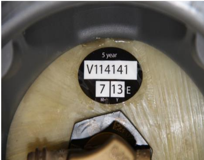
Picture4-2 Example requalification marks on pressure vessel
