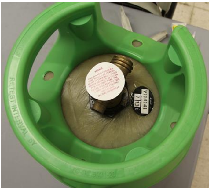
Picture 4-3 Example requalification marks on pressure vessel
