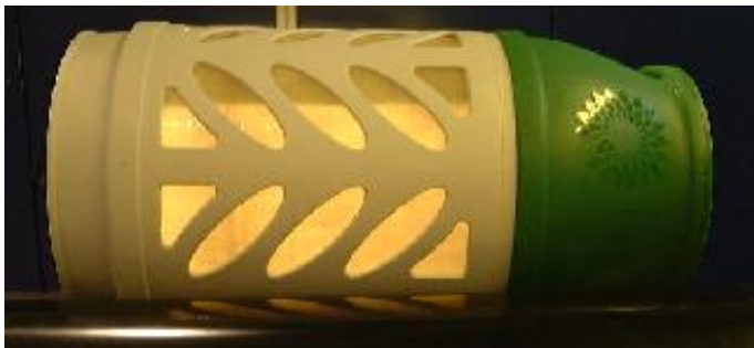
Picture 4-2 - Use of a strong back-light to inspect the cylinder. In this case, the remaining LPG in the cylinder is clearly visible.
