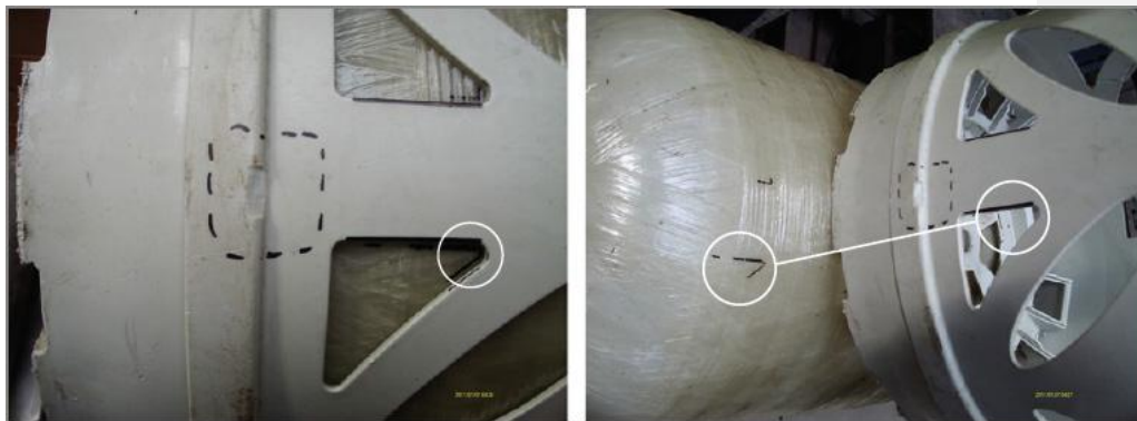
Picture 3-2 Marking on casing and pressure vessel – before and after casing removal
