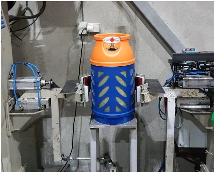
Picture 5-2 Example of cylinder clamping device.
