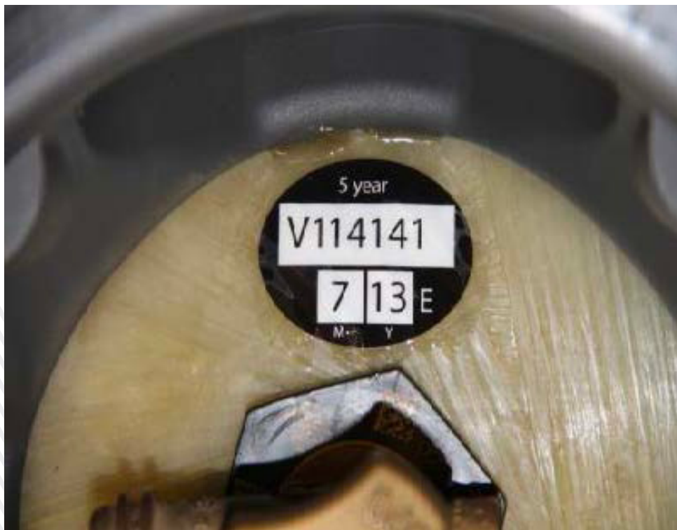
Picture 4-3 Example requalification marks on pressure vessel
