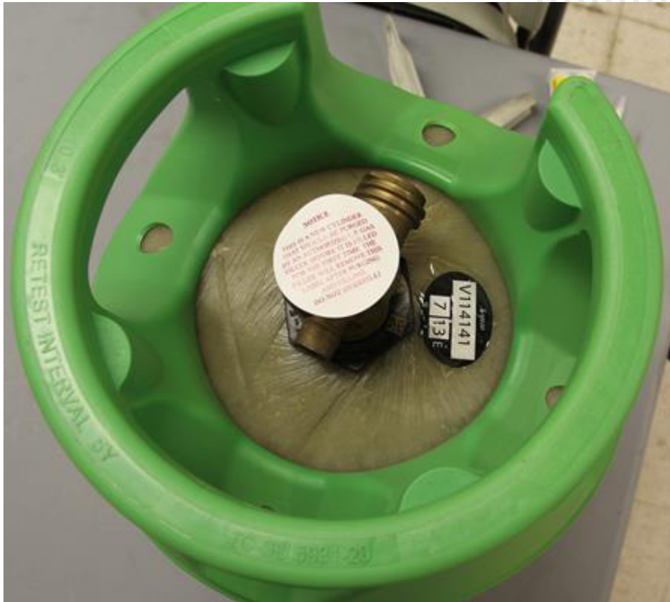
Picture 4-2 Example requalification marks on pressure vessel
