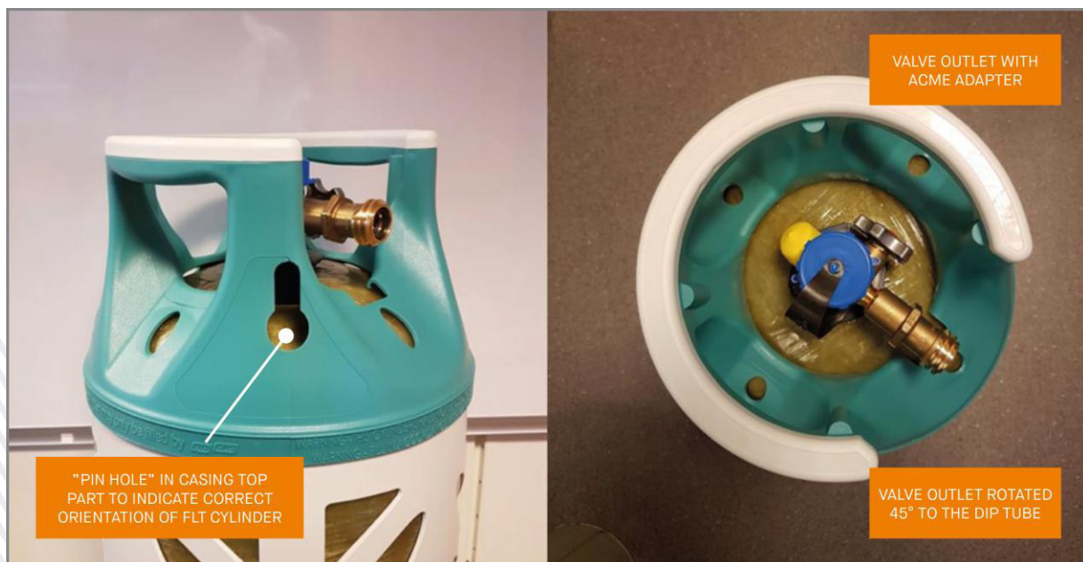
Figure 6-3 - FLT multivalve. The pin hole or keyhole shall be oriented so that the locator pin on the forklift truck is positioned in the pin hole. This ensures liquid withdrawal of the LPG.
